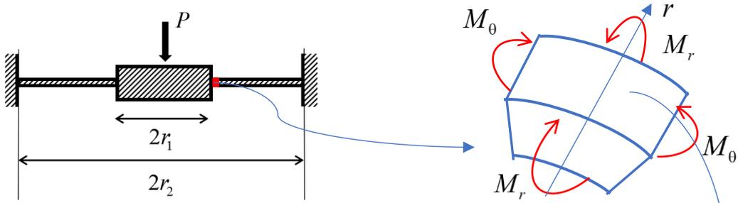
$$M_r(r_1) = P \cdot \bar{M}_r(r_1) = 0,156P, \quad M_\theta(r_1) = P \cdot \bar{M}_\theta(r_1) = 0,047P,$$
