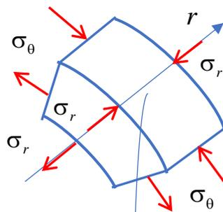
$$\sigma_r(r_1) = -\frac{6M_r(r_1)}{h^2} = -\frac{6 \cdot P \cdot \bar{M}_r(r_1)}{h^2} = \frac{0,156P}{h^2} = -5,841 \cdot 10^4 P,$$
